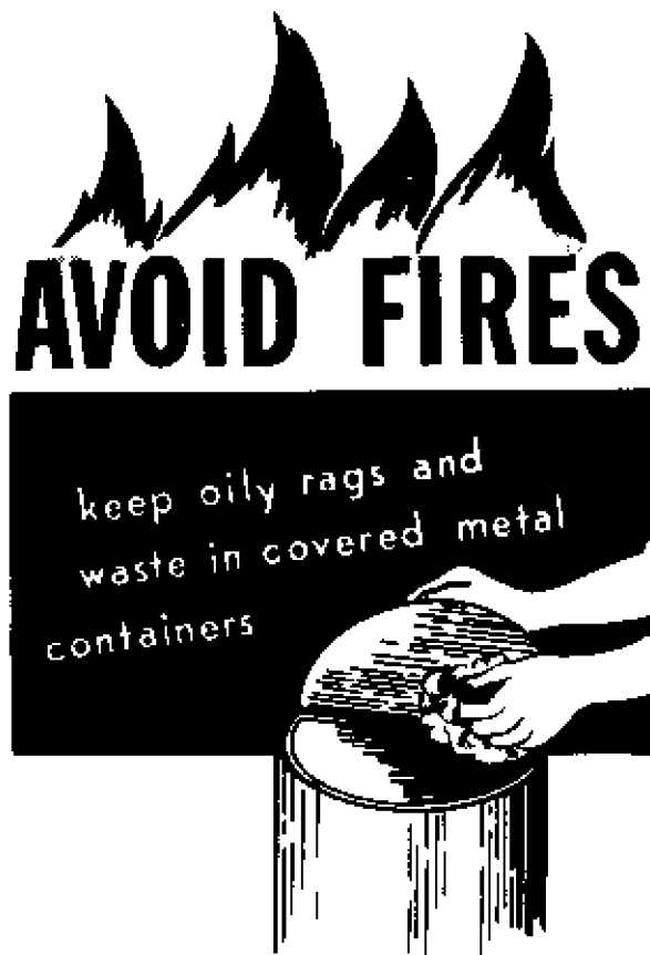
FIGURE 3-28 Combustible Waste, Separate Containers
